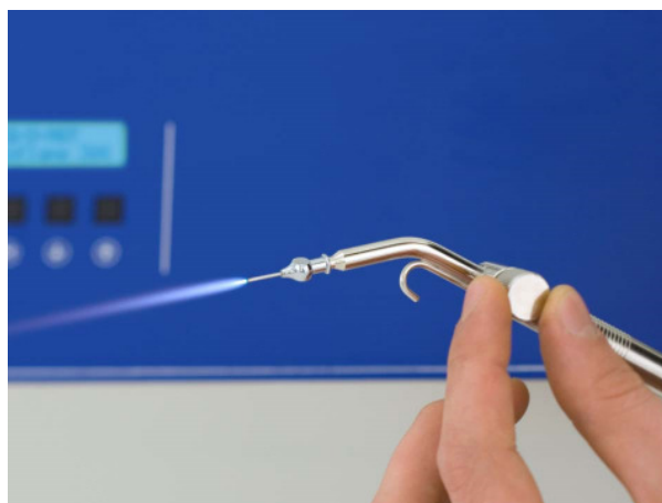
Figure 5.4. Regulation of the flame size with the valve on the burner handle
